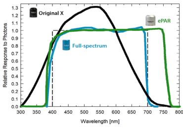
Mean **spectral response** measurements of six replicate Apogee MQ-210X (black), MQ-650 (green), and MQ-510 (blue) series quantum sensors compared to traditionally defined PAR 400-700 nm (dotted).
